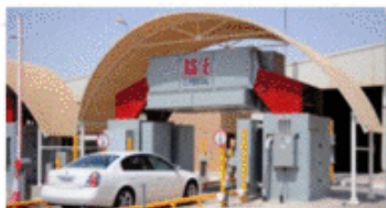
Z Portal®: Multi-view, multi-technology vehicle screening system for passenger vehicles, trucks and cargo
